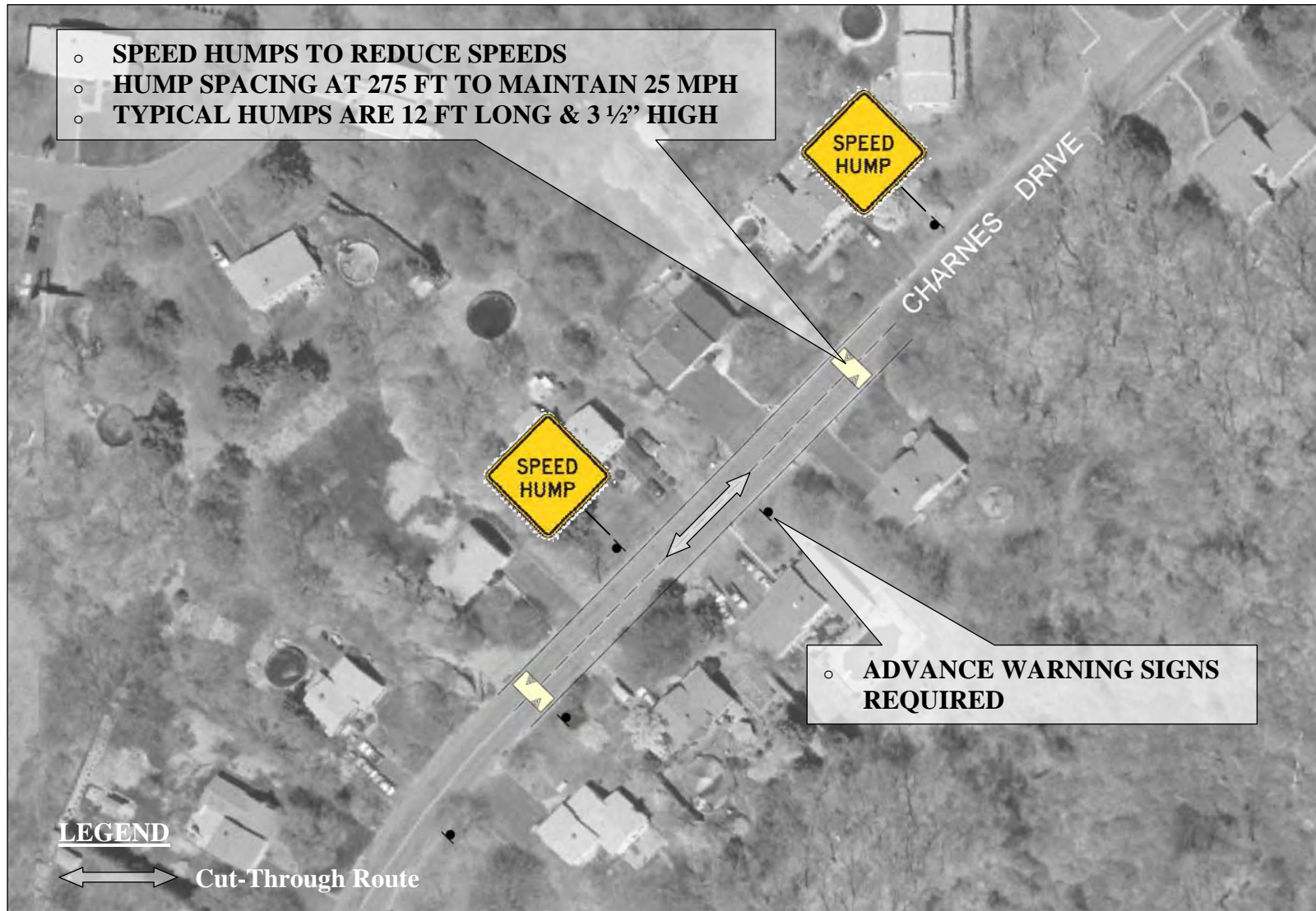
FIGURE 4-12. TRAFFIC CALMING EXAMPLE: SPEED HUMPS ALONG CHARNES DRIVE
